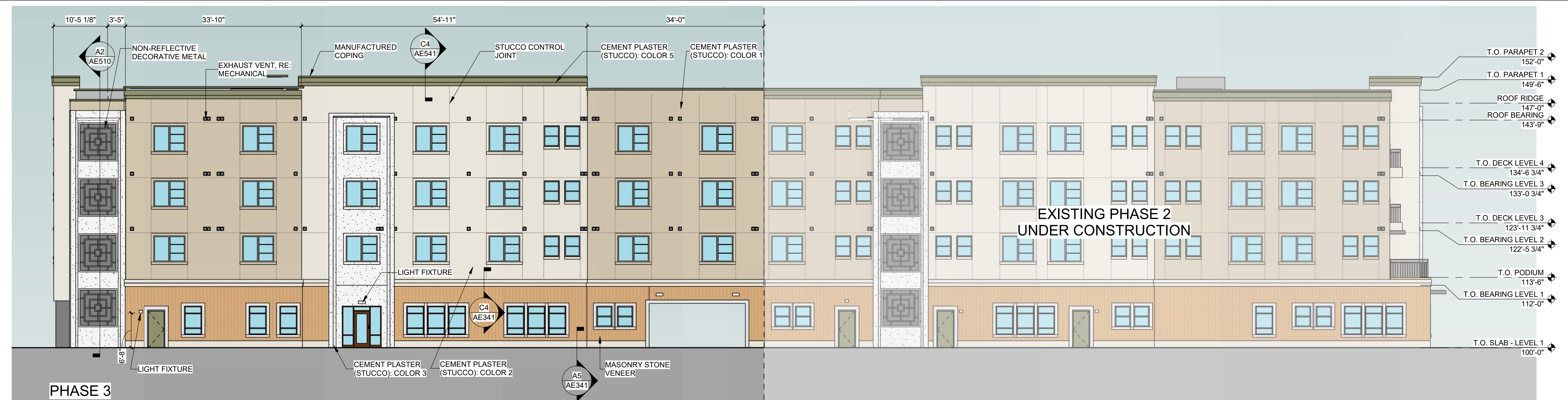
C1 WEST ELEVATION - OVERALL 3/32" = 1'-0"
